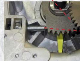
**Externally adjustable stop screw** prevents from manual overriding of the closed position.
