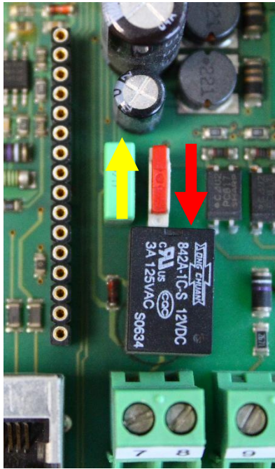
Figure 2: Slide switch for selecting the interface
