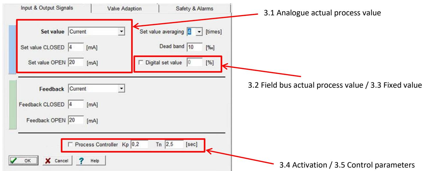
The setting for the set value and the actual process value must be in the same value range. Different settings are not possible.
