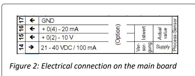
Figure 2: Electrical connection on the main board
