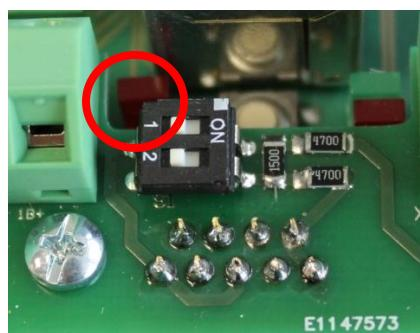
LED Off: Switches off in case of successful commissioning and correct start of the fieldbus.
