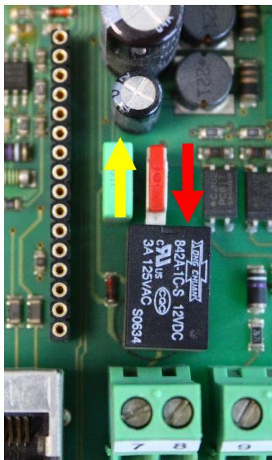
On the mainboard inside the actuator there is a slide switch for selecting the interface (see Figure 5).
