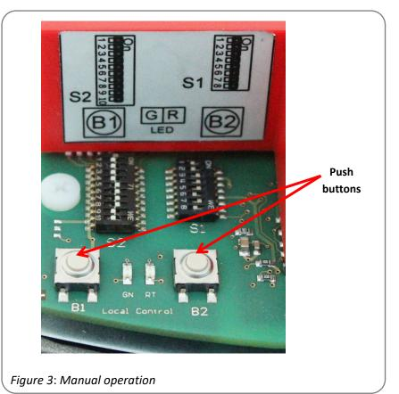
For commissioning the actuator during adjustment work (valve mounting and end position adjustment), an electrical manual override by means of a push-button is available (see 12.6 Manual operation).
