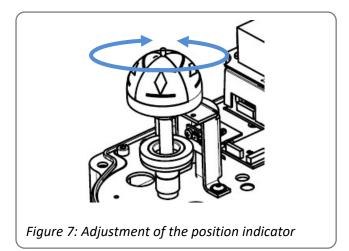
The position indicator is a two-coloured half ball turning under a transparent dome with blackened quarter segments.
