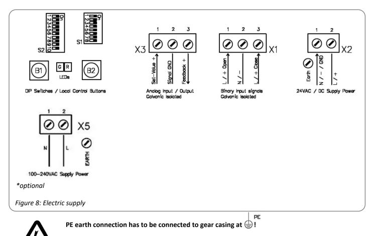
Ensure that all connecting cables are stripped to the correct length so that they are protected against electric shock.
