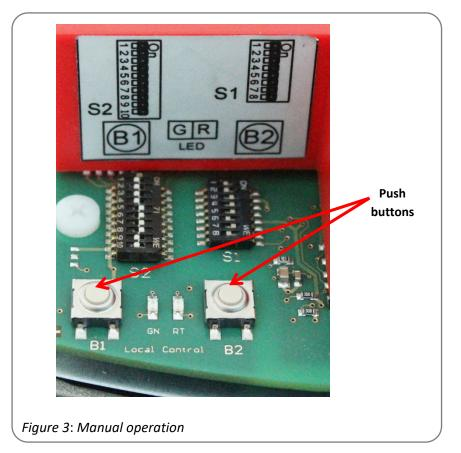
For commissioning the actuator during adjustment work (valve mounting and end position adjustment), an electrical manual override by means of a push-button is available (see 12.7 Manual operation).
