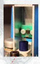
Contactless, non-wearing travel detection with Hall sensor for exact positioning
