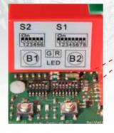
Manual operation with push buttons or handwheel. Parameter setting via **DIP** switches
