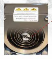
**Integrated power spring** for fail safe function in case of loss of power supply, either extending or retracting actuator stem
