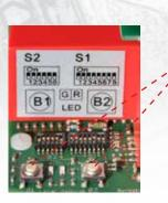
**Manual operation with** push buttons. Parameter setting via **DIP** switches
